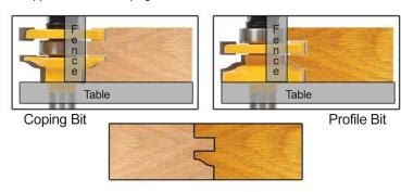
When using thinner stock, the top cutter should be situated at least 1/8" down from the top of the stock. Any less than 1/8" would likely result in a flimsy joint.
