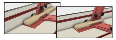
Install featherboards in the router table and route a piece of scrap material. Test the fit with one of the rails. Adjust the bit height or fence depth if the joint isn't aligned properly. Now route the inside edges of the rails and stiles with the stock face down. Refer to the rail and stile setup guide for instructions on adjusting the joint's fit.
