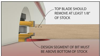
Set the coping bit in the router table. Place a piece of scrap material face down on the table to compare with the bit's height. Adjust the bit up or down until you reach the desired height, as long as the design segment of the bottom blade is above the bottom of the stock. The top blade should remove between 1/8" and 1/4" of material, and should never be below the top face of the stock.
