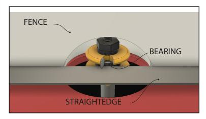
Set the fence with a straightedge placed against the bit's bearing. Move the fence forward until it touches the straightedge. Lock the fence in place.
