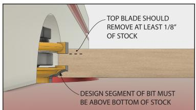
Set the coping bit in the router table. Place a piece of scrap material face down on the table to compare with the bit's height. Adjust the bit up or down until you reach the desired height, as long as the design segment of the bottom blade is above the bottom of the stock. The top blade should remove between 1/8" and 1/4" of material, and should never be below the top face of the stock.
