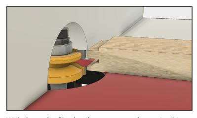
With the ends of both rails cut, remove the coping bit from the router and insert the profile cutter. You'll need one of the rails to set the bit height. Adjust the bit up or down until the slot cutter is aligned with the tenon in the end of the rail. Set the fence with a straightedge as a guide, just like you did in Step 3.
