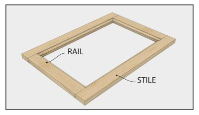
Choose a width for the stiles and rails. Somewhere between 2" and 2-1/2" is common for cabinet doors, but you can use any width you like. Just be sure there's enough material for the profile cutting-depth plus 1" for structural strength.
