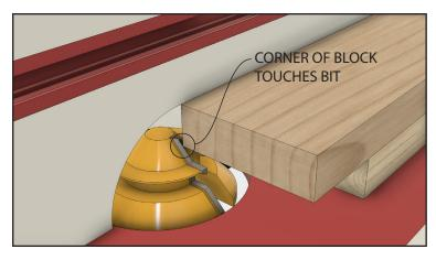
To get the fence depth just right, place a piece of stock on the router table with a scrap block on top. Extend the scrap slightly past the end of the stock. Butt the stock and scrap block against the fence. Adjust the fence until the corner of the scrap block just touches the bit.
