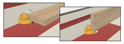
Run two pieces of scrap material through the router and test the lock-miter's fit.
