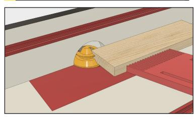
With the bit height and fence depth set correctly, route your stock. To make a four-sided column, route both edges of the front and back pieces face down. Then route both edges of the sides with their faces against the fence.
