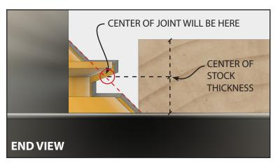
Install the bit in the router table and adjust the height so that the center of the joint aligns with the center of the stock's thickness.
