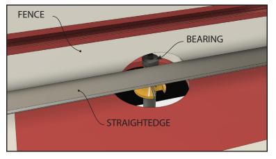
The fence should be flush with the bearing on top of the router bit. Place a straight edge against the bearing and pull the fence forward. When the fence and bearing are aligned, lock the fence in place.
