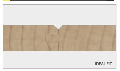
Route one edge of a piece of scrap equal in thickness to your stock. Test the joint's fit and move the bit up or down to correct any misalignment.
