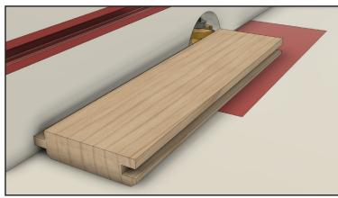
Each piece of stock that will be sandwiched between two others should be routed on two edges. Route the tongue on the edge opposite the groove. Remember to route the material face down for wainscoting or face up for v-notched flooring.
