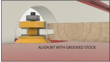
Remove the v-groove cutter and replace it with the tongue-cutting bit. Set a piece of the grooved stock on the router table and use it to adjust the bit height. Move the bit up or down until it appears to be aligned with the groove. The fence depth does not need to be changed.
