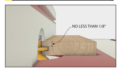
Insert the v-groove bit in your router table. Place a piece of stock on the table and adjust the bit height so that the top edge of the groove cutter is no less than 1/8" from the top face of the stock. You must have at least 1/8" of material between the groove and the face of the stock for structural integrity.
