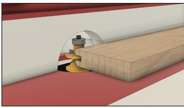
If you're going to make v-grooved wainscoting, route your stock face down. To create v-notched flooring planks, route the stock face up. Use feather boards to keep the material pressed against the fence and router table surface.
