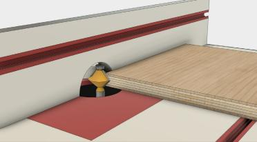
Cut the groove in your plywood or MDF parts. Feed the work at a slow and steady pace. Because the bit leaves sharp points at the top and bottom of the work piece, you may want to attach a guide block to the top of your material with double-sided tape. Any flat, straight piece of material will work and will give you a cleaner cut.
