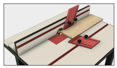
For the cleanest cuts and crisp edges, use a feather board to hold the stock to the router table's surface, and another to press the work into the fence. Feed segments face up for 6-sided objects at a slow and steady rate. A push stick will provide maximum control and will keep your hands at a safe distance from the router bit.
