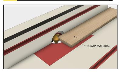
When your bit height and fence are properly adjusted, run a test cut on one edge of a piece of scrap the same thickness as your stock. Be careful to run the piece face up or face down according to the table below. Test the joint's fit.
