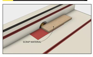
Run a piece of scrap material through the router and test the joint's fit. If the bit height and fence depth are correct, you're ready to route.
