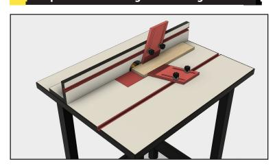
Run each segment through the router table face down. For the best results, use feather boards to keep your work pressed tightly against the table and fence. Feed slowly, and use a push stick to keep your hands at a safe distance from the bit.
