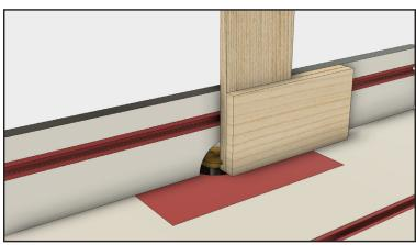
Route each drawer side with the material standing on its edge, using a push block for safety and stability. The drawer parts are now ready for assembly.
