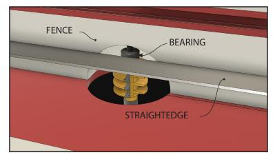
The fence should be flush with the bearing on top of the router bit. Place a straightedge against the bearing and pull the fence forward until it's flush. Lock the fence in place.
