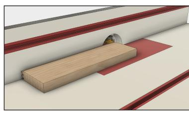
Make the first cut. Use a coping sled or miter gauge if you're going to make an end-to-end joint. Install feather boards to cut an edge-to-edge joint.
