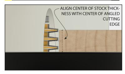
Install the bit in your router table and place a piece of stock on the table to compare with the bit height. Adjust the bit up or down so the angled portion of one of the finger cutters is aligned with the center of the stock.
