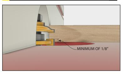
Install the bit in your router table and adjust the height for the coping cut. Place a piece of the stock you plan to route on the router table to help you gauge the height. Move the bit up or down until the top edge of the slot cutter is at least 1/8" above the tabletop.
