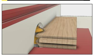
When the bit height is properly set, route the stiles and rails. Run the stock through the router face down.
