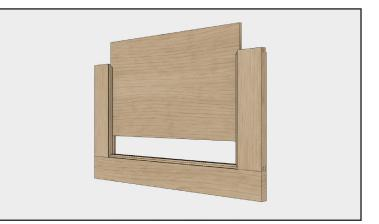
Install the second rail and slide the panel in place.
